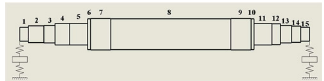
Fig. 2 Model of the rotor-bearing assembly to be analysed
