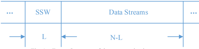
Fig. 1. Frame Structure of the communication system
