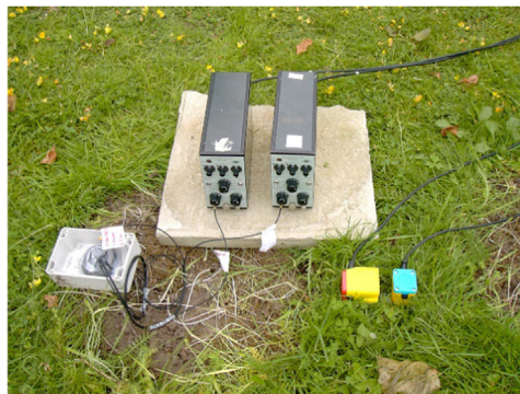
Fig. 13. Measurement setup showing geophones and PVDF wires.
