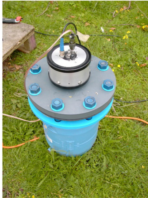
Fig. 12. Shaker mounted on the plastic end-plate.
