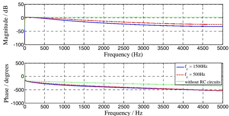
(a) Responses of different low-pass filters and the DSP delay
