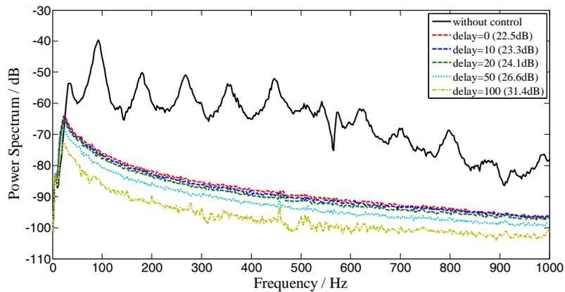
Figure 3. Predicted control performances with different delays of primary path
